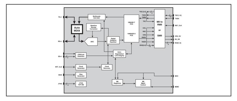
The Broadcom<sup>®</sup> BCM5226 is a single-chip device containing six independent Fast Ethernet transceivers. Each performs all the physical layer interface functions for 100BASE-TX full-duplex or half-duplex Ethernet on Category 5 twisted-pair cable and 10BASE-T full or half-duplex Ethernet on Category 3, 4 or 5 cable. Each port may also be configured for 100BASE-FX full or half-duplex transmission over fiber-optic cabling when paired with an external fiber-optic line transceiver.
